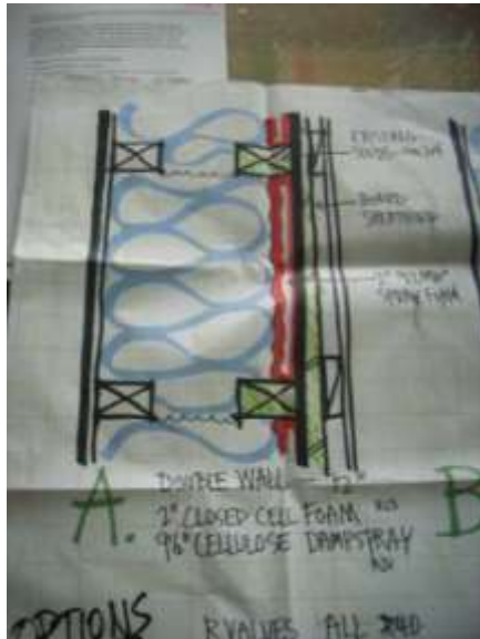
Double Wall – Flash Coat and Cellulose
