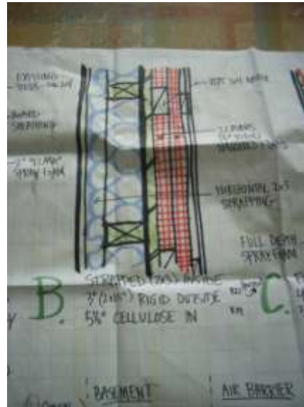
Strapped Inside – Foam or Cellulose In, Rigid Outside
